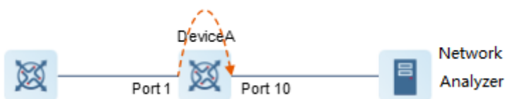
Figure 3-7 Operating Principle of Port Mirroring
