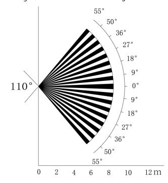
The vertical detection distance of the sensor is 2 m–10 m, 1 m–14 m or 1 m–12 m. Figure 7-2 Vertical detection distance
