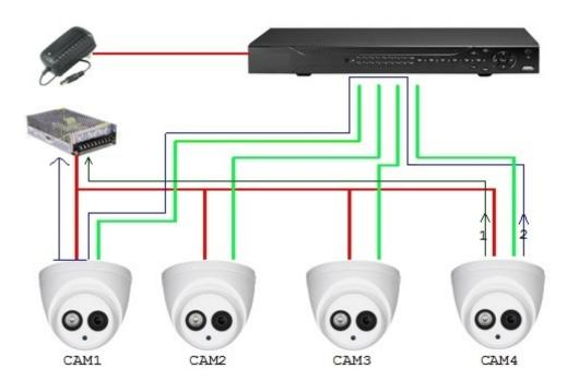
There are two paths for the power output of CAM4, return path 1 and return path 2. Reflow 2 first flows to CAM1, and then flows to the power supply from power supply ground of CAM1. In this way, the reflow of power supply ground CAM4 affects the video ground of CAM1, resulting in interference stripes on the screen. And CAM4 also interferes with CAM2 and CAM3.
