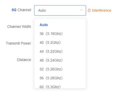
The camera mode does not support independent channel settings. After the channel at the NVR end is adjusted, the camera end automatically changes its channel to be the same as the NVR end.
