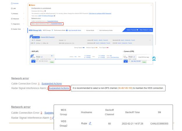
According to the information about the WDS group and back-off channel in the alarm record, check whether the current working channel in the WDS group (group 2 in the example) is consistent with the back-off channel. (See <u>Displaying WDS Group Information</u>.) If so, manually switch the channel to a non-dynamic frequency selection (DFS) channel. For the setting method, see <u>Channel settings</u>.
