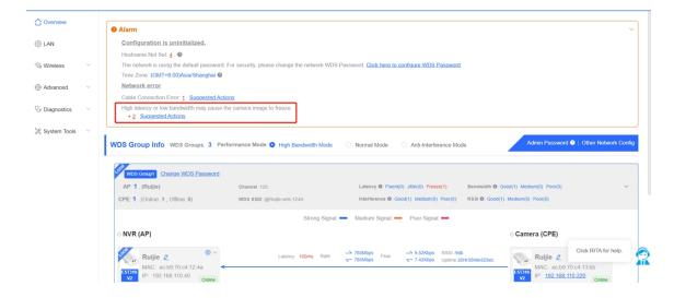
High latency or low bandwidth may cause the camera image to freeze.
