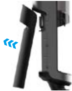
6. Open the back cover very hard with tweezers.
