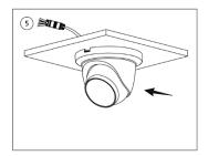
Figure 3-8 Cable going through the side cable tray
