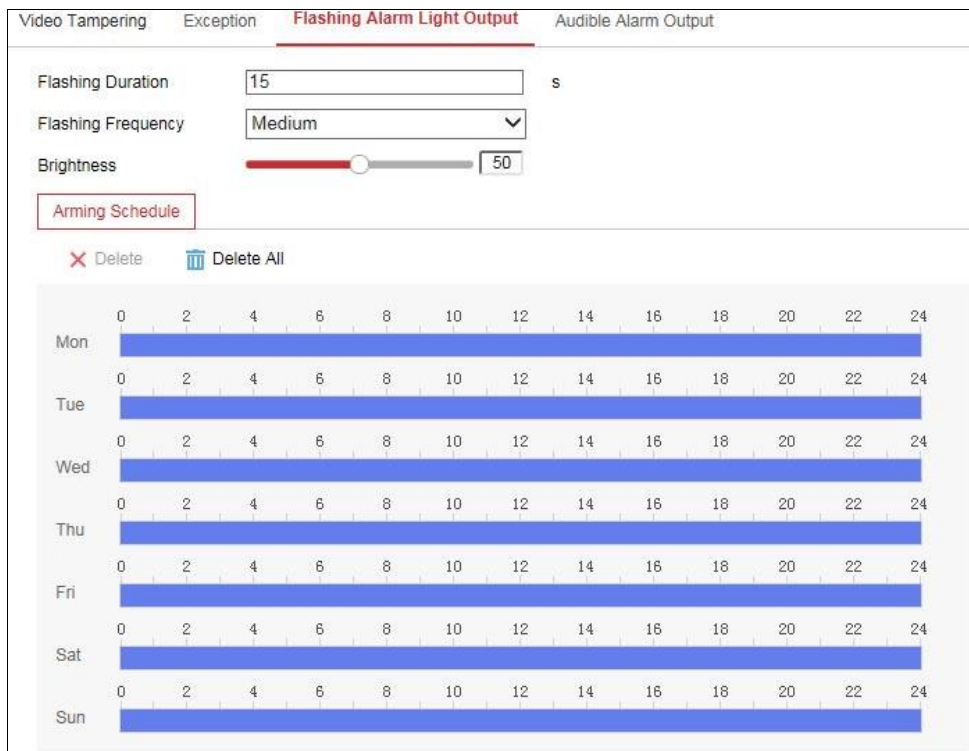
Figure 10-9 Flashing Alarm Light Output Settings
