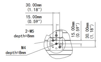
Detail A Engineering installation screw hole Size ratio 1:2 4 positions in total
