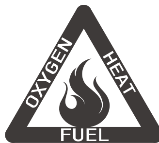
Figure 1 Three Necessary Factors for Explosion
