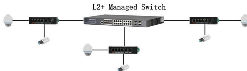
Figure 1-2 Typical networking scene of 8-Port Switch
