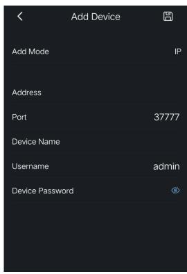
Step 3 Enter Address (IP address of the door station (VTO)), Device Name, and Device Password.
