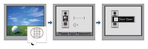
When the Door Station is in standby, Press "#"
