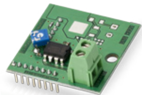
EA2 - audio output module with amplifier
