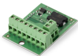
EPGM8 - hardwired PGM output expansion module
