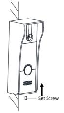
Figure 4-7 Securing the Door Station
