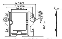
Figure 4-1 Wall Mounting Plate
