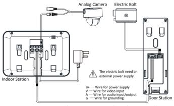
Figure 3-3 Wiring 1 (1 Door Station and 1 Indoor Station)
