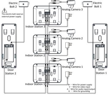
Figure 3-5 Wiring 3 (2 Door Stations and 3 Indoor Stations)
