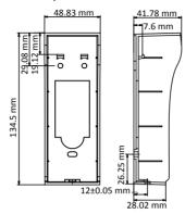
Figure 4-4 Wall Mounting Shield
