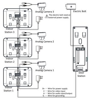
Figure 3-4 Wiring 2 (1 Door Station and 3 Indoor Stations)
