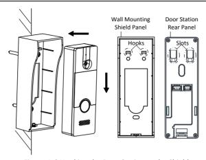
Figure 4-6 Hooking the Door Station to the Shield
