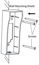
Figure 4-5 Installing the Shield
