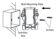
Figure 4-2 Installing the Plate
