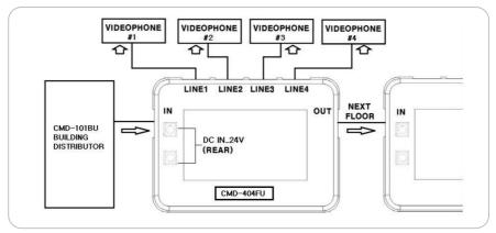
CCTV / LOBBY → Building distributor(CMD-101BU) → CMD-404FU(1<sup>ST</sup> FLOOR) → CMD-404FU(1<sup>ST</sup> FLOOR) → CMD-404FU(2<sup>ND</sup> FLOOR) → ... → MODUME VIDEO PHONE
